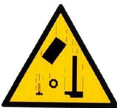
Caduta materiali Watch for falling materials
